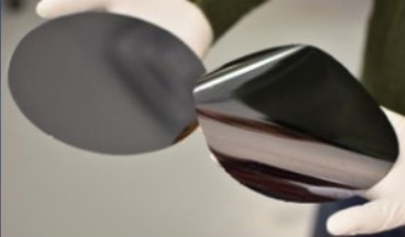
Microlink Devices' 150mm diameter ELO foil Foil is <30 μm thick and flexible
