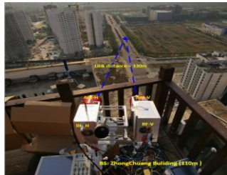
Fig. XIII-6. THz field trial, 2 x 2 polarization-MIMO system
