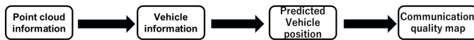
Fig. IX-6. The developed mechanism to prepare radio quality maps from point cloud data which is acquired by the millimeter wave radar.
